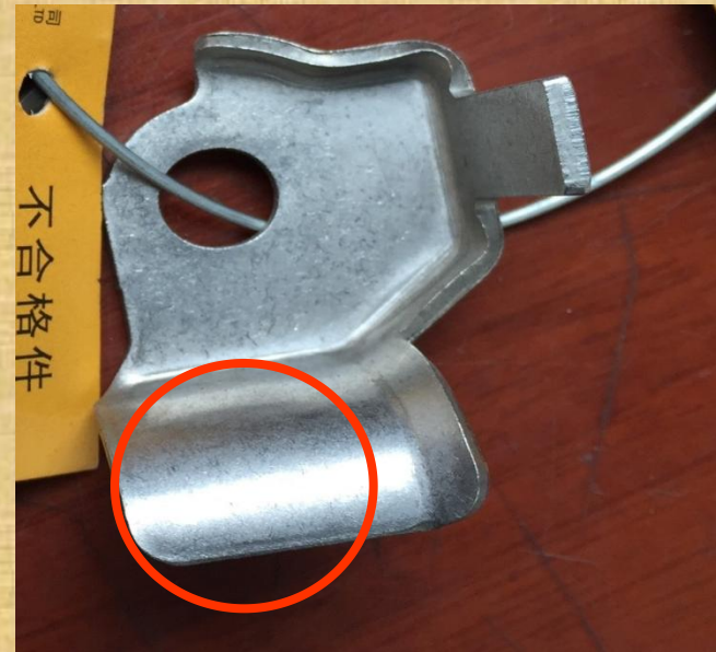
16268-518YL-2 Missing Dot
