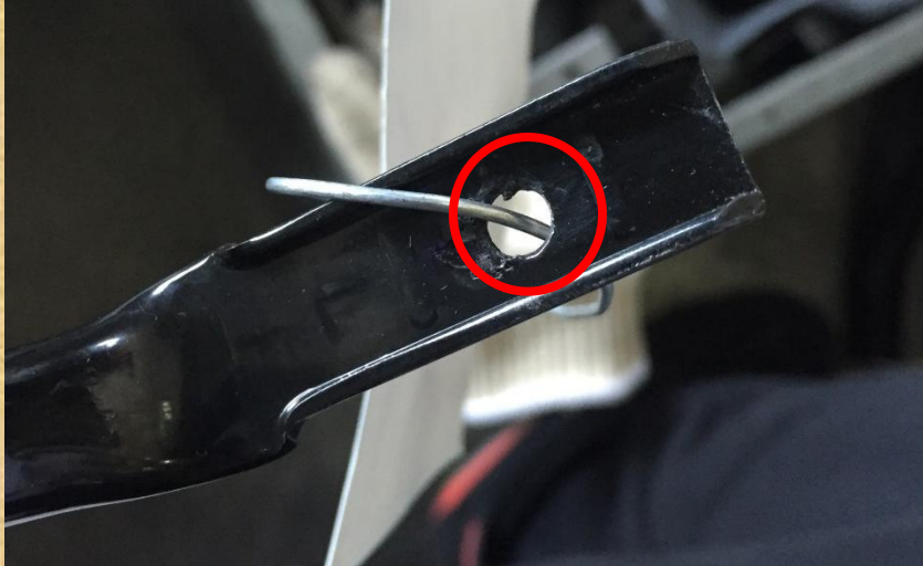
29PG 161 The edges of the hole have burrs
