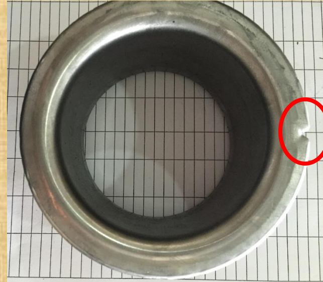
8RD 505 336 Surface Cracks
