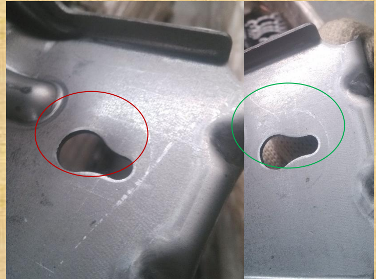
44591 Elongated Hole Deformation
