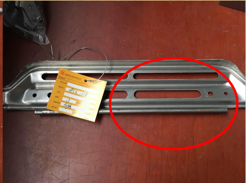
19LG 128 Surface rust
