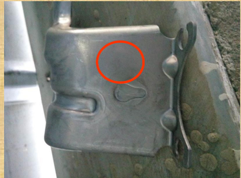
44591-1 Side hole not fully punched
