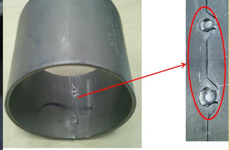
8RD 505 335 The inner wall has burrs
