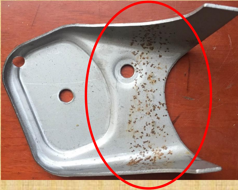
8RD 505 367/368 Surface rust
